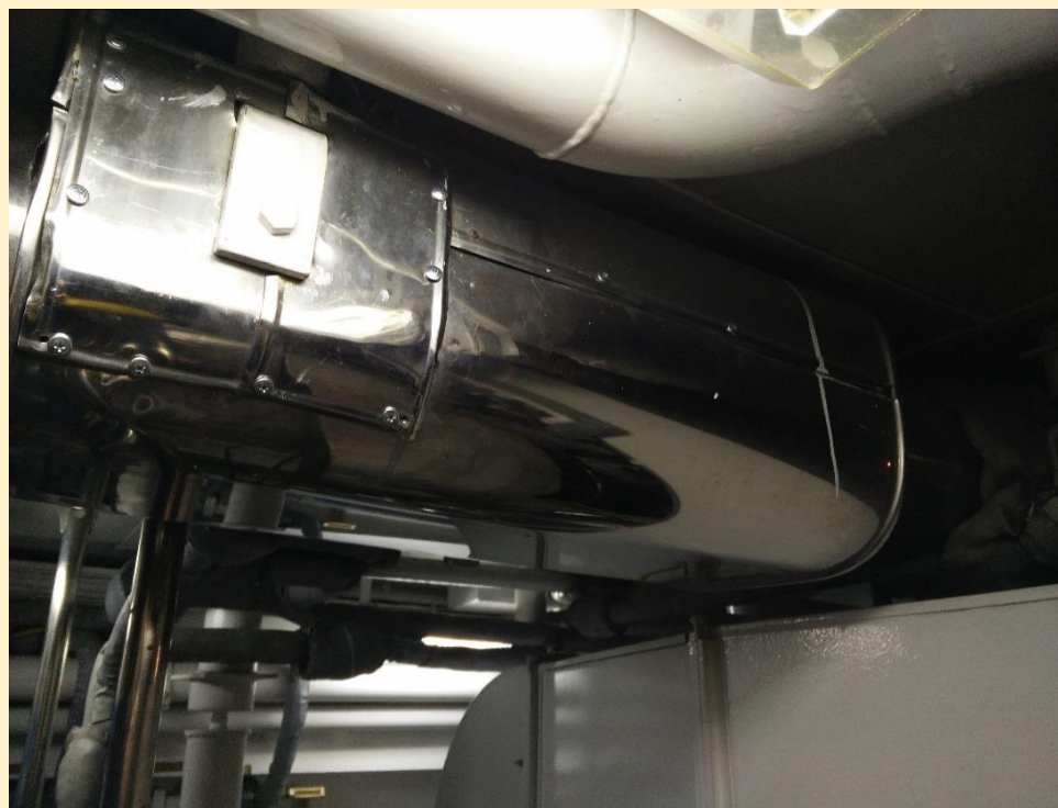
INOX STEEL METAL PLATING AT EXHAUST PIPE IN MAIN ENGINE WITH INSPECTION DOOR
