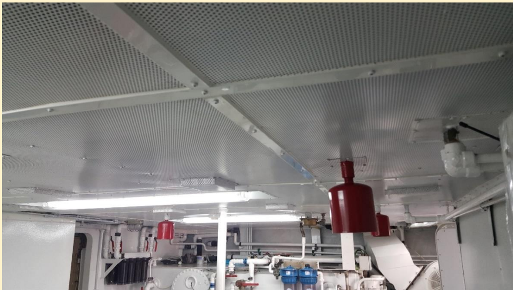
A-60 SOUND INSULATION AT ENGINE ROOM WITH METAL CLADDING OF PERFORATED STEEL SHEET
